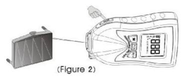
2.Locating a hot spot aim the thermometer outside the area of interest, then scan across with up and down motions until you locate the hot spot.(please turn on the laser to for accurate measuring)
